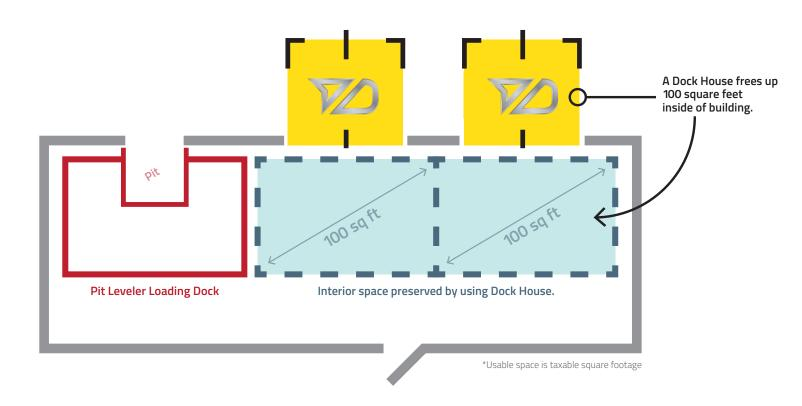
When a facility attaches Dock House modular loading docks to its exterior, the inside of the building is much cleaner and a significant amount of floor space is preserved. In fact, each Dock House loading dock installed outside a facility will preserve 100 sq. ft. of internal floor space.
