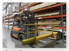
**REMOVE:** Forklift slides into integral fork pockets to easily lift barrier section
